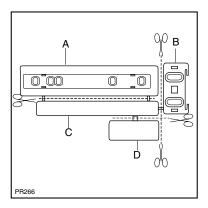
Place guide (A) on the inside part of the furniture door, in the upper and lower position as shown in the figure and mark the position of external holes. Having drilled the holes, fix the guide with the screws supplied.
